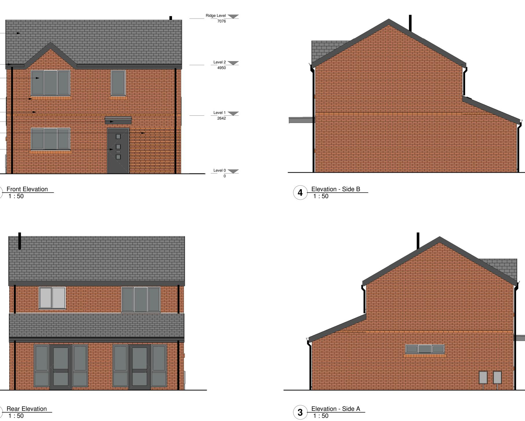
Russel Grampian Slate Grey. -concrete single lap roof tiles and system
